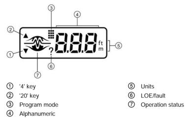
2. It then defaults to the **Run mode**, which is the measurement reading of the distance from the transducer face to the material level in the units indicated as shown:
